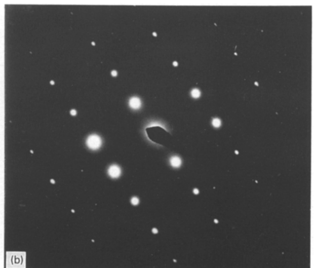
Figure 9 Selected-area diffraction patterns obtained from a needle-shaped titanium boride particle, which can be indexed as orthorhombic TiB. (a) [\bar{1}01]_{\text{TiB}} ; (b) [1\bar{2}1]_{\text{TiB}} ; (c) [\bar{1}11]_{\text{TiB}} .
